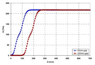
Figure 2: Longitudinal variation of field gradient between magnets.
