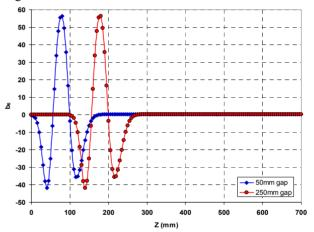
Figure 3: Longitudinal variation of b<sub>6</sub> between magnets.
