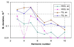
Figure 4: Normal  $b_n$  and skew  $a_n$  random errors in 5 Nb<sub>3</sub>Sn TQ and 8 NbTi HGQ models.
