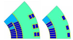
Figure 4: 2D finite element thermal model of NbTi IRQ.
