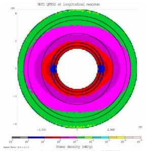
Figure 3: Power density isocontours in QFEX2 magnet.
