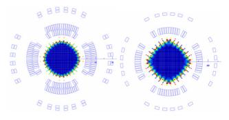
Figure 2: 4-layer and 2-layer QD0 magnet cross-sections.
