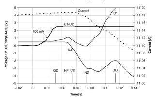
Figure 2: Voltage signals at the start of the quench. Note that the data acquisition time is 5 ms, the signal U1-U2 is limited at 250 mV, and the signals U1 and U2 are filtered values.
