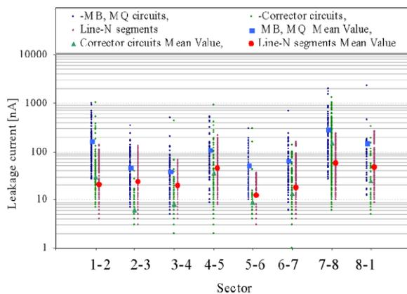
Figure 4: Leakage current versus circuits for all sectors.
