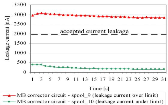
Figure 6: Leakage current in corrector magnet circuits.
