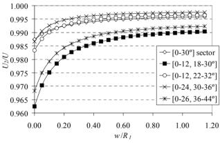
Figure 2: Ratio between the magnetic energy produced by the main harmonic (n=2) and the total energy versus  $w/R_I$  for five different sector coils.
