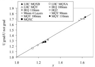
Figure 4: Increase of magnetic energy due to grading as a function of *x* as defined in (16).
