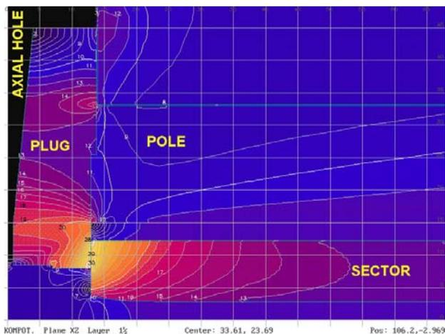
Figure 6: Magnetic field distribution in the vertical section of the magnet centre region with the small diameter of plug axial hole.
