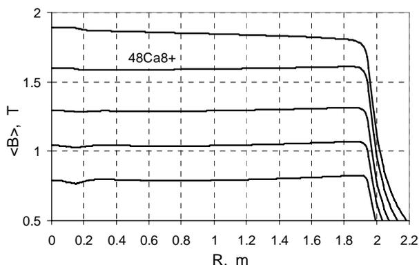
Figure 3: The results of final calculation of U400R cyclotron average magnetic field.
