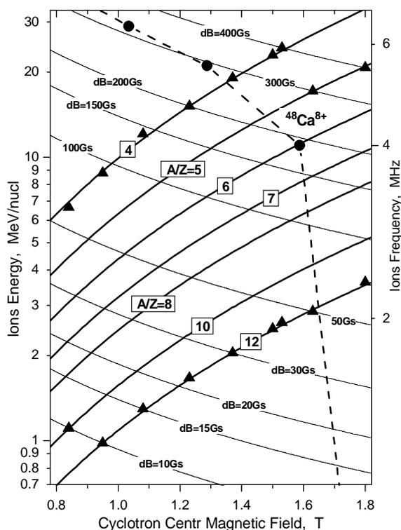
Figure 1: The working diagram of the U400R cyclotron.
