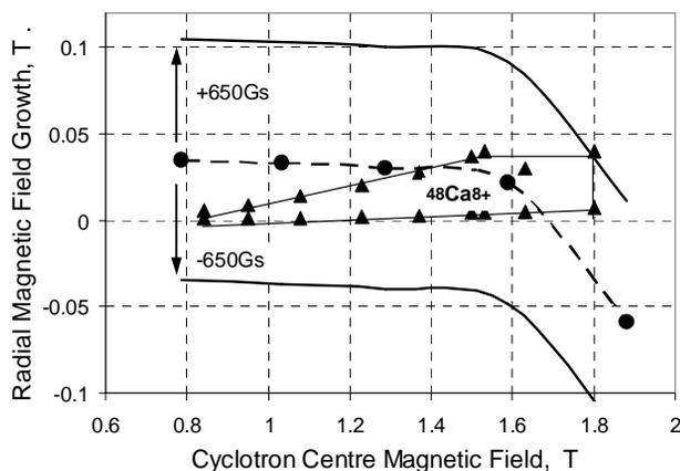
Figure 2: The working diagram area (triangle) and the real magnetic field behaviour (line with circles) of the U400R cyclotron.
