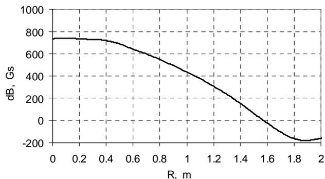
Figure 4: The sum contribution of the ten radial trim coils at the average magnetic field level 1.8T.
