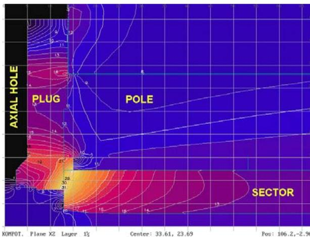
Figure 7: Magnetic field distribution in the vertical section of the magnet centre region with the big diameter of plug axial hole.
