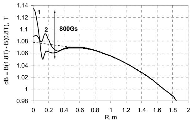
Figure 5: The difference of the average magnetic field at the high, 1.8T and low, 0.8T levels.
