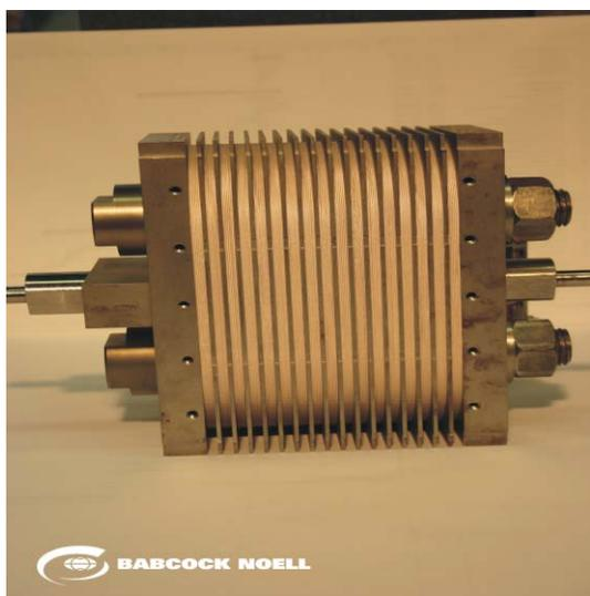
Fig. 2 Nb<sub>3</sub>Sn Undulator mock-up before heat treatment.
