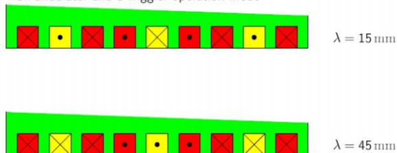
Fig. 4 The Undulator / Wiggler SCUW with an electrically switchable period length from 15 mm to 45 mm. The period length is switched by reversing the current in the yellow marked windings.
