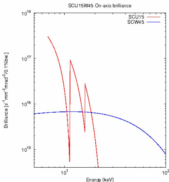
Fig. 5 Calculated brilliance of a 15/45 mm period length undulator /wiggler for the storage ring ANKA. The stored current is assumed to be 200 mA.
