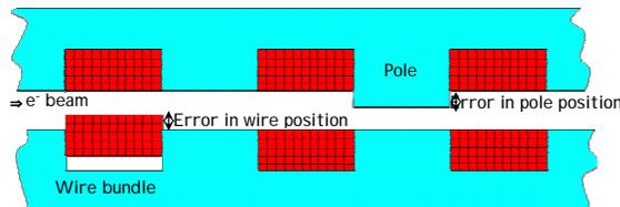
Fig. 3 Possible mechanical errors contributing to the phase error in a superconducting undulator: errors in the pole position and errors in the position of the wire relative to the pole.
