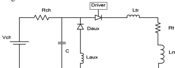
Figure 5: Simplified septum pulser electrical circuit.
