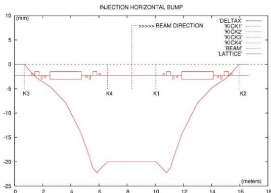
Figure 2: SESAME injection horizontal bump scheme.
