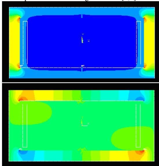
Figure 3: Magnetic field density, Bx(lower) and By(upper) of the kicker magnet.
