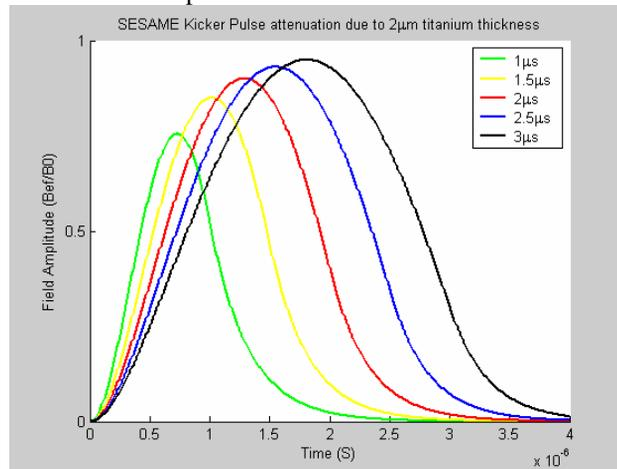
Figure 4: Field attenuation for various pulse durations.
