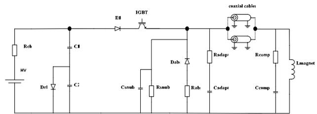
Figure 6: Kicker electrical pulsed circuit
