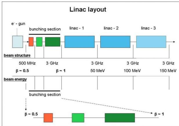
Figure 1: The schematic layout of the TPS-linac bunching structure.
