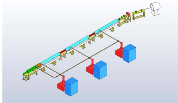
Figure 2: The general layout of the 150 MeV linac.
