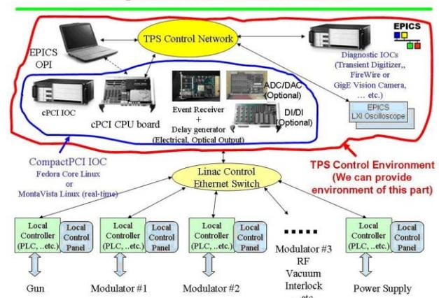
Figure 3: The proposed interface and control environment.
