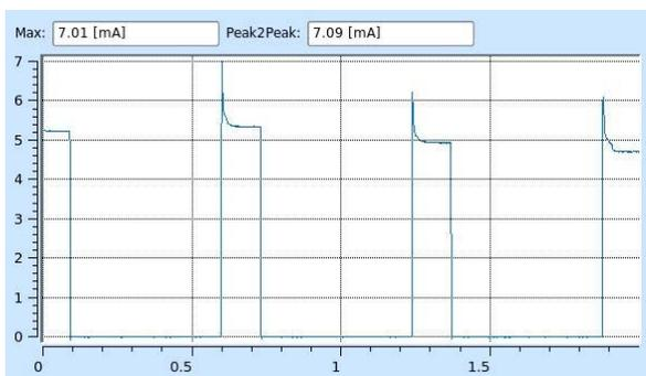
Figure 2: Booster beam current, ramping & extraction.
