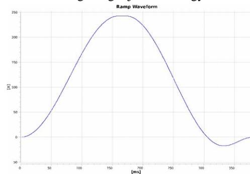
Figure 3: Bending power supplies ramping curve.
