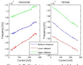
Figure 4: Drift in betatron tune and sidebands
