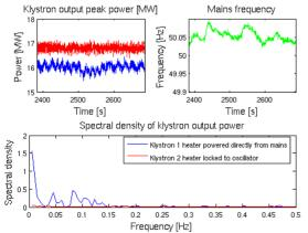
Figure 1: Comparison of klystrons with heater powered by mains (blue) and locked to the timing oscillator (red). Slow power beat is absent for the synchronised heater.
