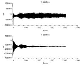
Figure 7: Turn-by-turn BPM measurement of kick following fine tuning of injection kickers. Maximum kicks are  $\pm 30 \ \mu m$  and  $\pm 140 \ \mu m$  in horizontal and vertical planes respectively.
