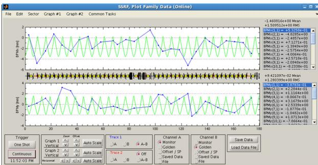
Figure 7: Booster closed orbit without correction.
