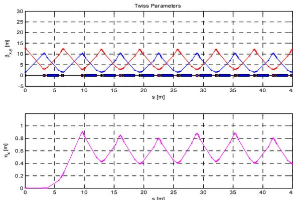
Figure 2: Twiss parameters of SSRF booster synchrotron. (One fourth of the ring is shown.)
