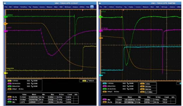
Figure 4: ICTs at LINAC and high energy transfer line. Left: LINAC ICT 1.332nC. Right: HT ICT 0.993nC.
