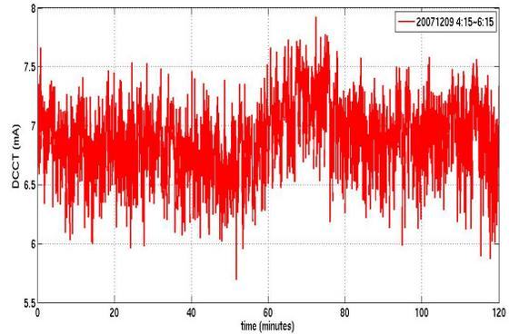
Figure 8: Current stability with multi bunch mode.
