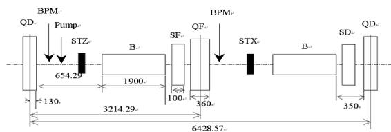
Figure1: Layout of one standard booster cell.
