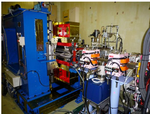
Figure 1: Photograph of the circular/linear polarized undulator with a fast switching orbit bump system.
