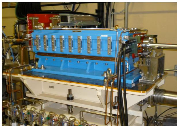
Figure 2: Photograph of the pulsed bending magnet as the most upper bend along the PF-BT installed in the 3<sup>rd</sup> switch yard of the linac tunnel.
