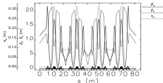
Figure 1: Optical functions in a super-period of TPS.
