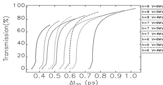
Figure 6: Transmission of photons through the slit vs of duration of radiation for various crab cavity parameters.
