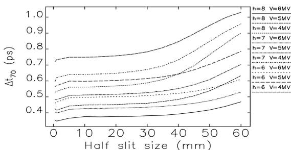
Figure 5: Duration of 70 % of central X-ray pulse as a function of slit size for various deflecting structure parameters.
