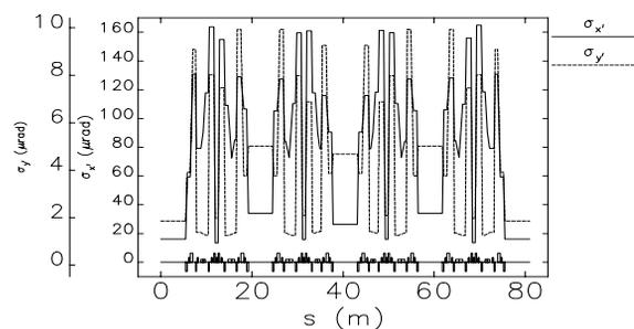
Figure 3: Transverse electron beam divergence in a super period of TPS.
