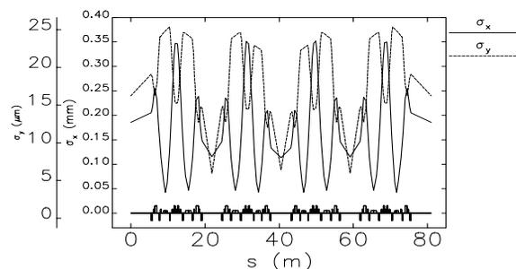
Figure 2: Transverse electron beam size in a super period of TPS.
