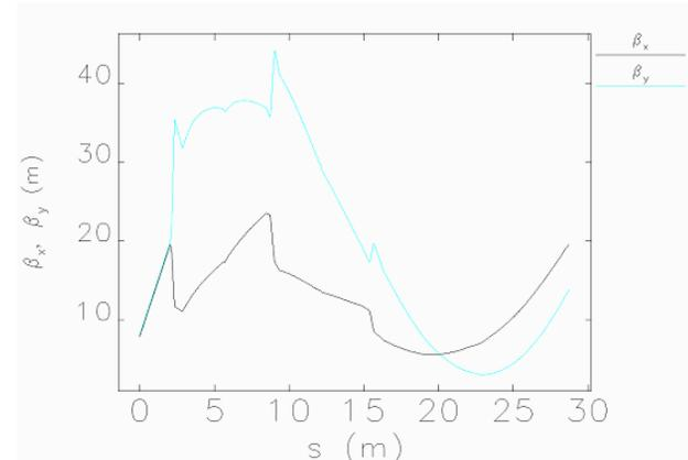
Figure8: Beta function of the linac.
