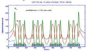
Figure 2: Lattice functions of the TPS lattice.
