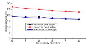
Figure 13: Dynamic aperture vs. chromaticity for the cases with hard-edge and soft-edge models.
