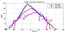
Figure 6: Dynamic aperture tracking for on-energy and off-energy particles at long straight center.
