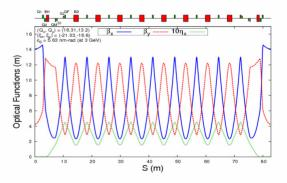
Figure 14: Lattice functions of the booster synchrotron.
