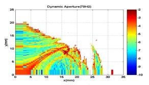
Figure 7: Dynamic aperture for on-energy particle (TRACY-2) at long straight center.
