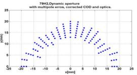
Figure 12: Dynamic aperture tracking for 10 sampling machines with multipole errors and corrected COD and optics. No chamber limitation in the simulation.
