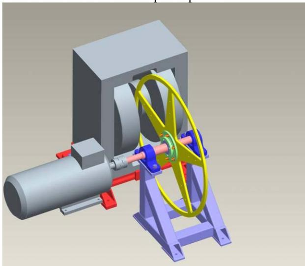
Figure 3. Target wheel test rig set up.
