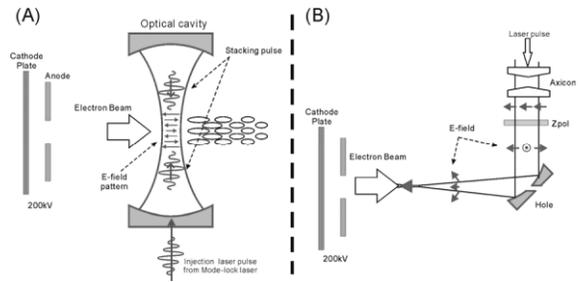
Fig.2: Schematic drawings of laser modulation using (A) optical resonator with focal waist and (B) z-direction polarized laser pulse.
