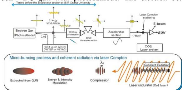
Fig. 1: Schematic drawing of considering scheme and laser Compton scattering with pre-bunched electron beam.
