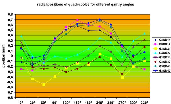
Figure 7: Radial positions of gantry quadrupoles.
