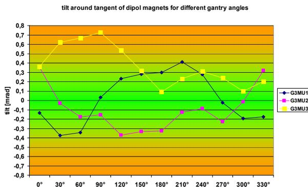
Figure 9: Tilt around tangent of gantry dipole magnets.
