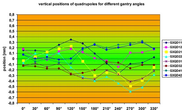
Figure 8: Vertical positions of gantry quadrupoles.
