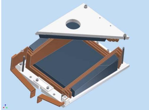
Figure 2: Cut through the bumper magnet indicating the three-turn coil and the ferrite.
