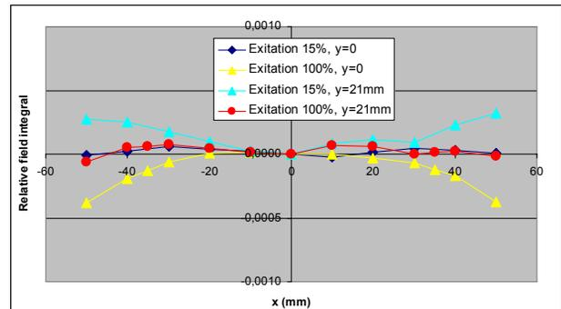
Figure 3: Relative field integral for one main dipole.
