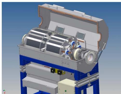
Figure 5: The RF cavity with the ceramic gap at the front.
