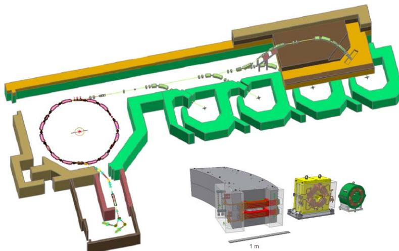
Figure 4: Layout of PT facility. The main synchrotron magnets are shown in the foreground with an enlarged scale.
