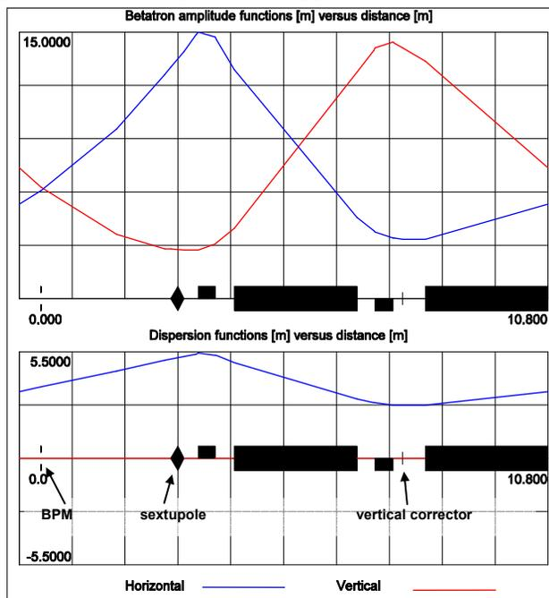
Figure 1: Lattice functions in one period of the synchrotron.
