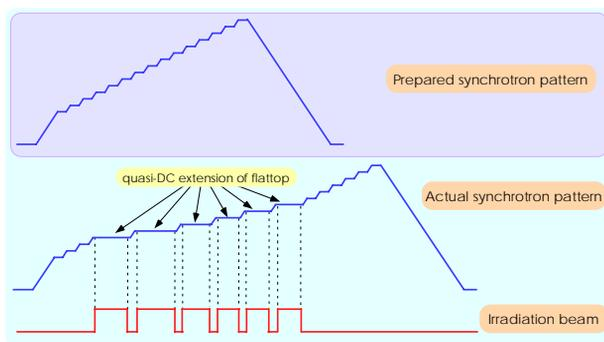
Figure 4: A schematic drawing of the synchrotron patterns for the multiple-energy operation with the quasi-DC extension of the flattop. The stepwise patterns show the current pattern of the main bending and quadrupole magnet of the synchrotron ring.
