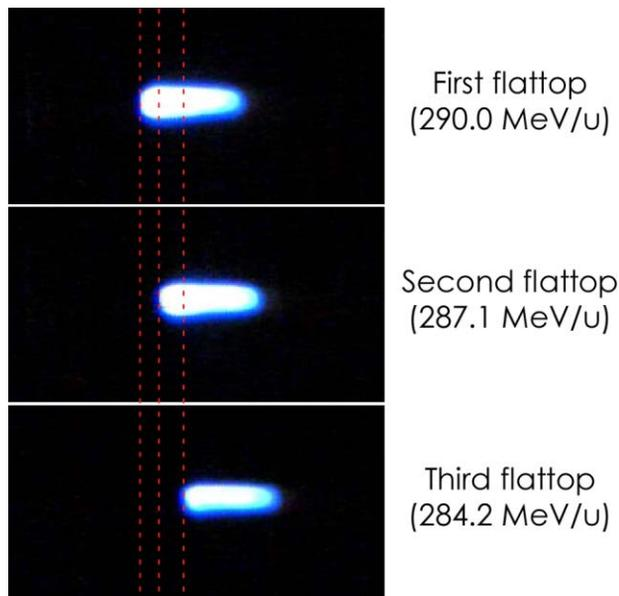
Figure 7: Pictures of a screen monitor. Three beam spots, corresponding to the respective beam energies, are clearly observed.
