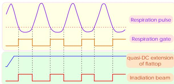
Figure 2: A timing chart of a respiration-gated irradiation using the quasi-DC extension of the flattop operation.
