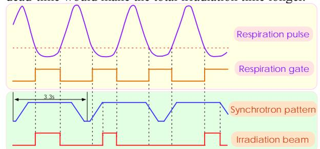
Figure 1: A timing chart of a respiration-gated irradiation.
