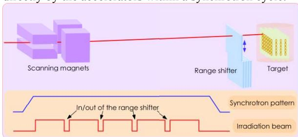
Figure 3: A schematic drawing of the quasi-DC extension of the flattop operation with a range shifter.
