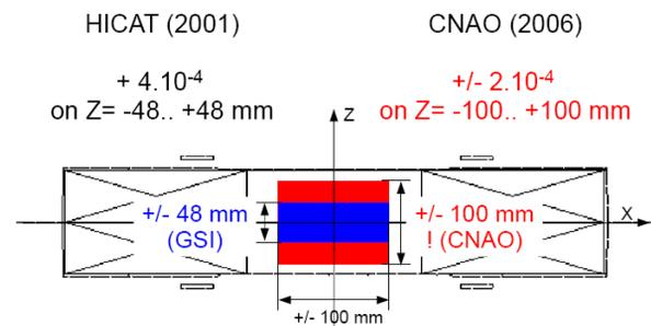
Figure 2: Specifications on integral field homogeneity
