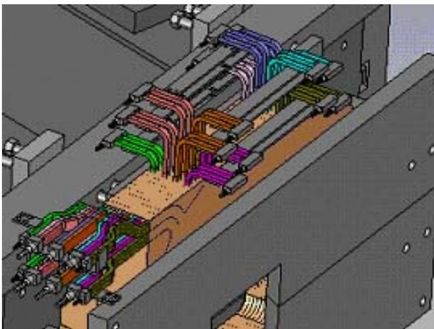
Figure 6: Bedstead end of the coil on the entrance side with current leads and cooling circuit busbars
