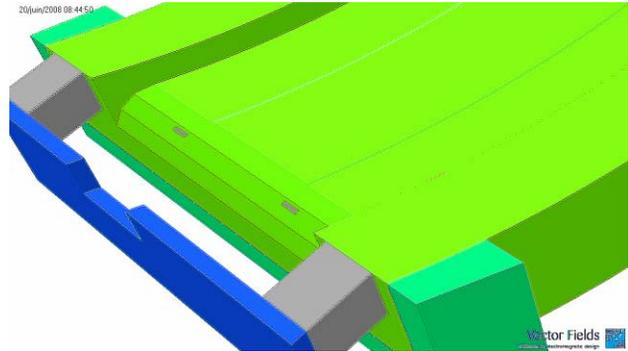
Figure 4: Detail of one of the edges showing the pole profile, the triple Rogowski, the pole slots (gray), the field clamp (blue) and the iron collar (water green).
