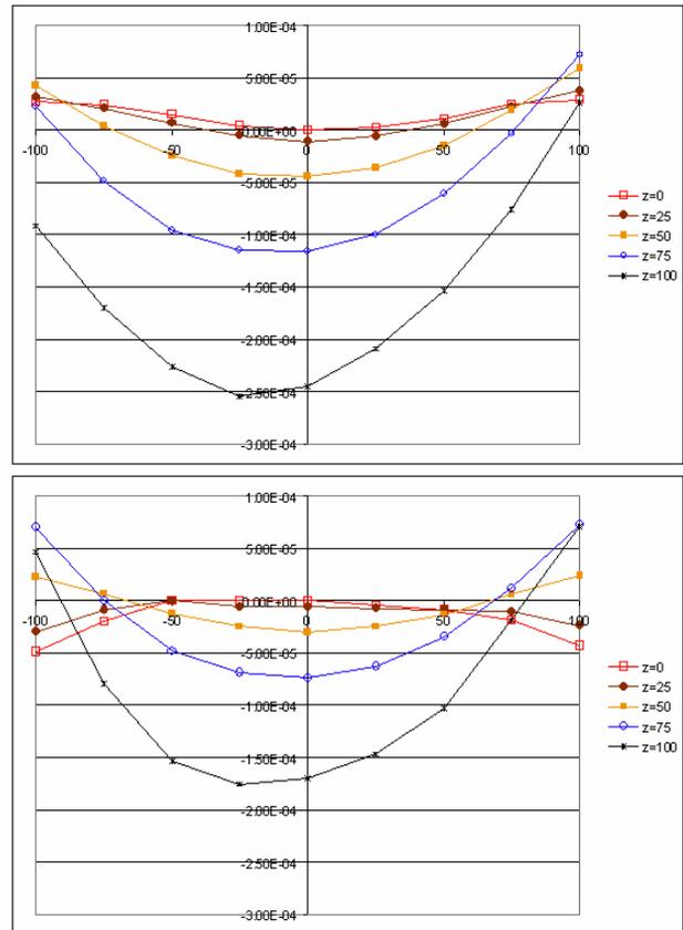
Figure 5: Comparison between the Integral field homogeneity versus radial offset in the original HICAT (top) and revised (bottom) designs in different axial planes at  $B_0=1.86$  T (nominal current).
