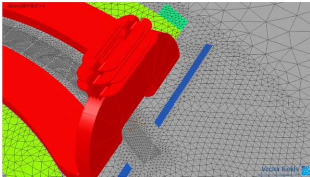
Figure 3: Bedstead end showing mesh density, subsections for mesh control and cooling busbars
