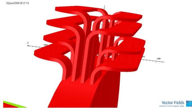
Figure 7: Detail of the modelling of the busbars
