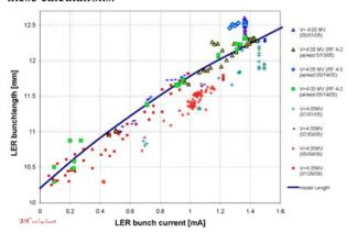
Figure 7: The LER bunch length as a function of current.
