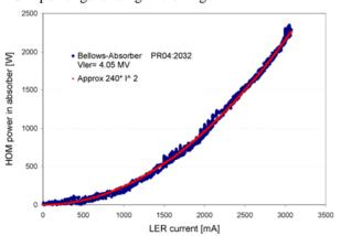
Figure 1: HOM power captured by the bellows absorber (blue diamond) and fitted quadratic function (red line)
