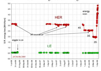
Figure 2: Synchrotron radiation energy losses in the PEP-II rings.
