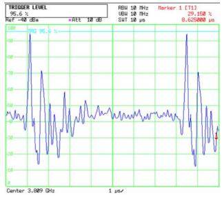
Figure 9: Transient at f=3.8 GHz.
