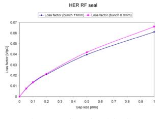
Figure 5: Loss factor of a sealed cavity.
