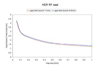
Figure 6: Electric field in the gap.
