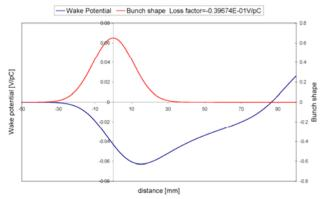
Figure 4: Wake potential of a 11 mm bunch.
