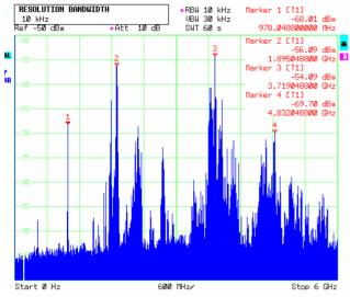
Figure 7: Single-bunch spectrum.
