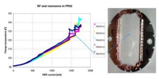
Figure 1: HER temperature resonances and omega seal.
