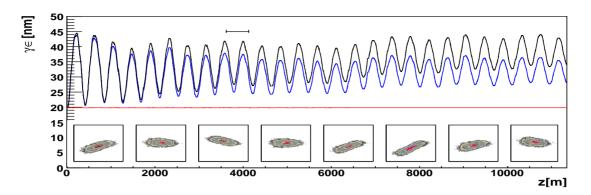
Figure 3: Coupler wakefield kicks: The projected emittance  $\gamma \epsilon_y$  along the main linac. The old coupler design is shown in black, the influence of the 1-2-1 steering in blue. The flat red line shows  $\gamma \epsilon_y$  for the new configuration. The additional small plots show the bunch in the *y*-*ct*-plane ( $-1mm \le ct \le 1mm, -20\mu m \le y \le 20\mu m$ ) in the middle (marked by a short black line) of the linac. The head of the bunch points to the right.
