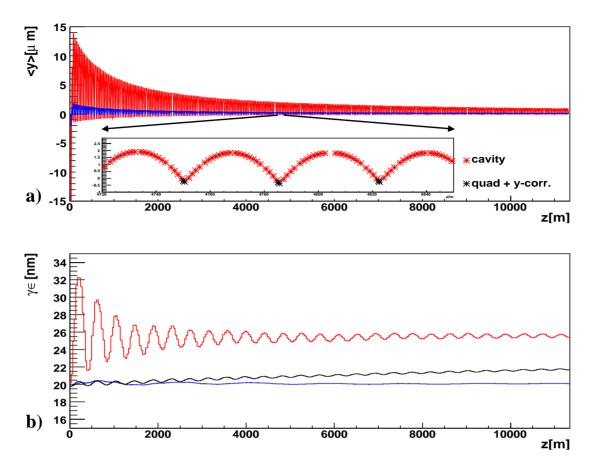
Figure 4: Coupler RF kicks: The new coupler design is shown in red, the old configuration in blue. The upper plot shows the trajectory  $\langle y \rangle$  along the main linac. The lower plot shows projected emittance  $\gamma \epsilon_y$  and the dispersion corrected emittance for the new coupler orientation in black.
