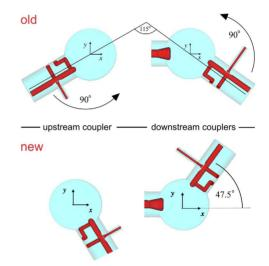
Figure 2: Relative orientation of couplers for the nominal (old) and the modified (new) design.
