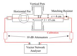
Figure 2: Setup of the impedance measurements.
