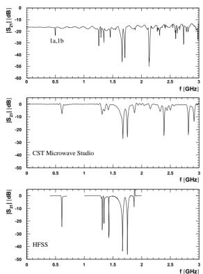
Figure 3: Comparison of the measured (top) and the simulated (middle and bottom) transmission coefficient  $|S_{21}|$  with all pots in retracted position ( $d_x = d_y = 40 \text{ mm}$ ).
