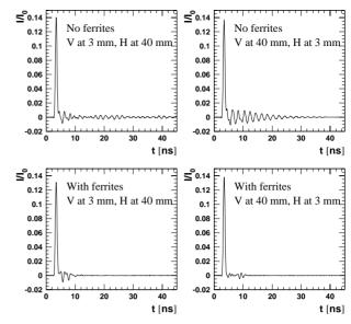
Figure 7: Transmission of a Gaussian pulse of magnitude  $I_0$  without (top) and with (bottom) ferrites for two different combinations of the horizonal (H) and vertical (V) pot distances from the wire.
