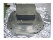
Figure 1: Left: the vacuum chambers of a RP unit accomodating the horizontal and the vertical pots and a Beam Position Monitor. Right: the pot with the thin window and a Ferrite collar (black).
