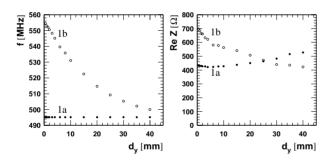
Figure 4: Frequency and impedance of the first double resonance as a function of the distance of the vertical pots from the wire, with retracted horizontal pot.
