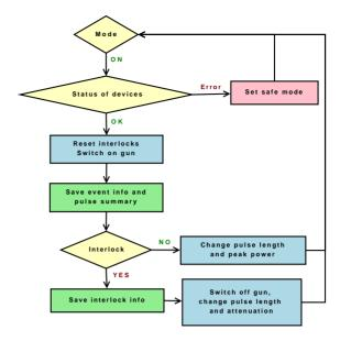
Figure 4: The conditioning logic
