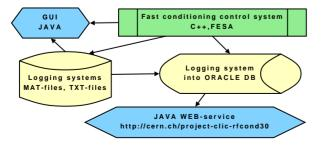
Figure 6: 30 GHz conditioning software infrastructure 06 Instrumentation, Controls, Feedback & Operational Aspects
