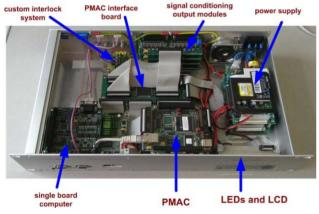
Figure 4: Inside of the microIOC-M-Box.
