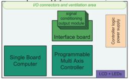
Figure 3: 3rd generation microIOC-M-Box.
