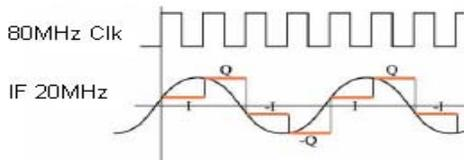
Figure 2: Digital IQ Demodulation.
