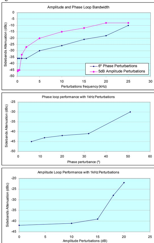
Figure 4: Bandwidth and ripples rejection of the loops.
