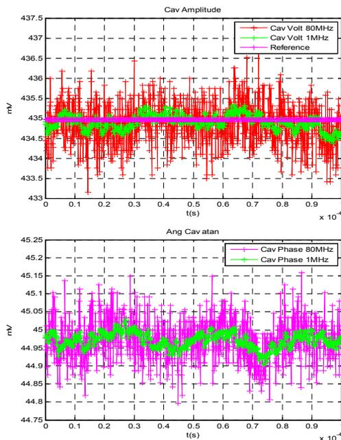
Figure 5: Loops resolution at high power (75kW).
