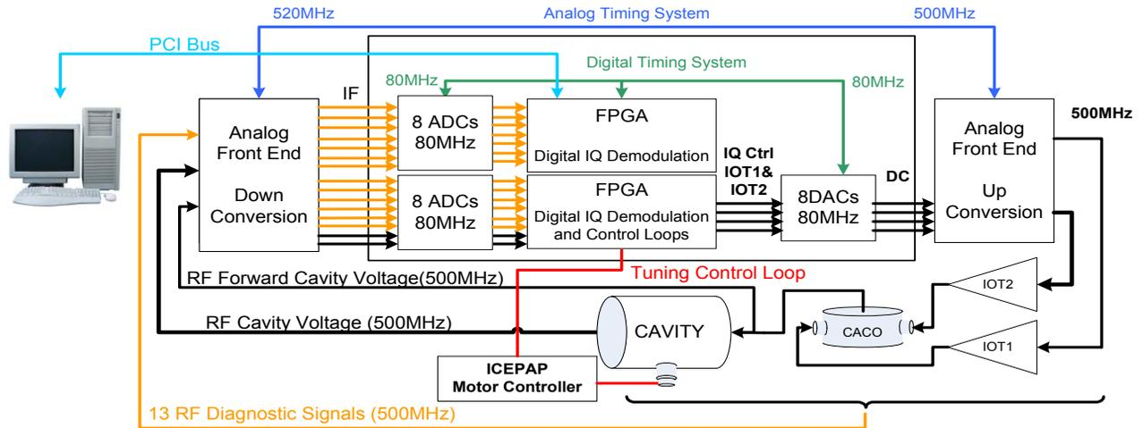
Figure 1: Digital LLRF Hardware Scheme.
