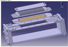
Figure 3: Drawing of the horizontal IPM.
