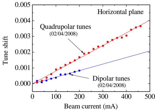
Figure 7: Measured dipolar and quadrupolar tune shifts in the horizontal plane. Lines indicate linear fits to the data.
