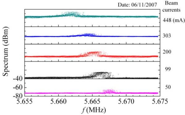
Figure 6: Responses of the vertical quadrupolar oscillations. Ten traces at each beam current were superposed.
