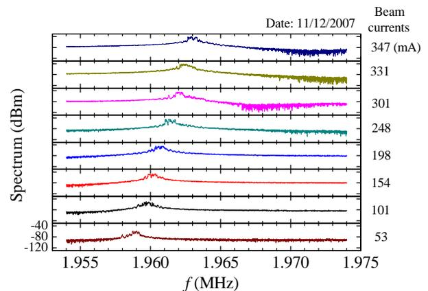
Figure 5: Responses of the horizontal quadrupolar oscillations.
