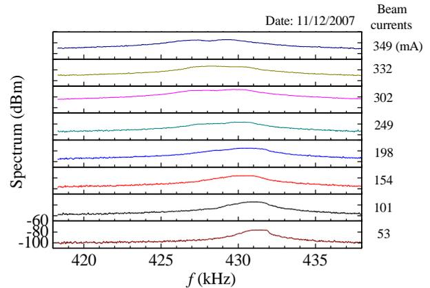
Figure 4: Responses of the vertical dipolar oscillations.
