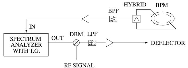
Figure 1: Setup for the dipolar tune measurements.
