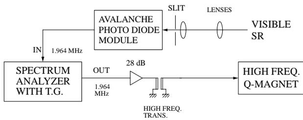
Figure 2: Setup for the quadrupolar tune measurements.
