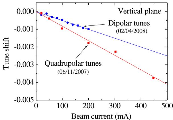
Figure 8: Measured dipolar and quadrupolar tune shifts in the vertical plane. Lines indicate linear fits to the data.
