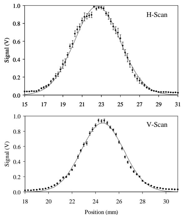
Figure 4: Typical profile measurement at LW14. Dots are measurement data and lines are Gaussian fitting.
