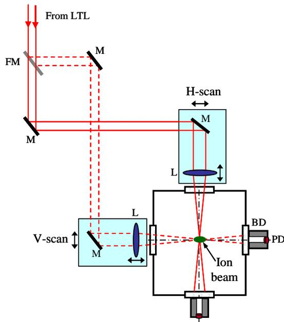
Figure 2: Schematic of laser wire station. L: lens ( $f=200$  mm), M: mirror, FM: flip-mirror, BD: beam dump, PD: photodiode.
