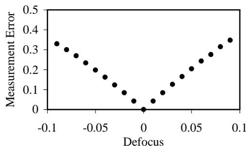
Figure 6: Calculated result of the beam size measurement error caused by the laser beam instability as a function of the lens defocus.
