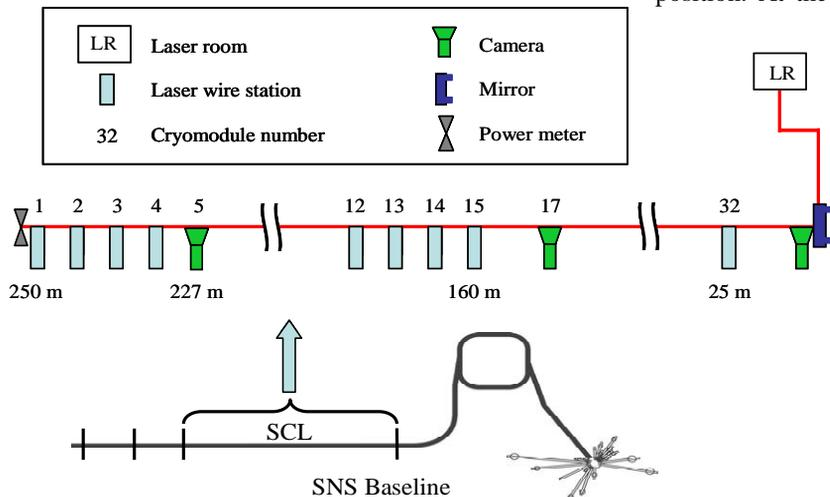
Figure1: Outline of the laser wire system installed in the SNS superconducting linac. Distances in the figure are from the laser room.
