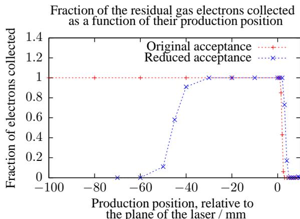
Figure 4: The longitudinal acceptance of the detector. Electrons collected from a non-zero production position correspond to background.
