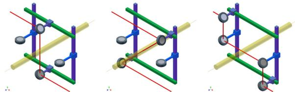
Figure 1: A schematic diagram illustrating how different projections of the ion beam (yellow) will be made by directing the laser beam (red) through it at different angles, guided by mirrors mounted on movable stages inside the vacuum vessel.
