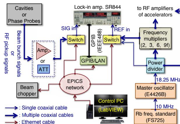
Figure 2: Schematic block diagram of developed monitoring system.
