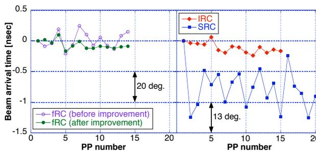
Figure 5: Isochronous condition of new cyclotrons in uranium acceleration.
