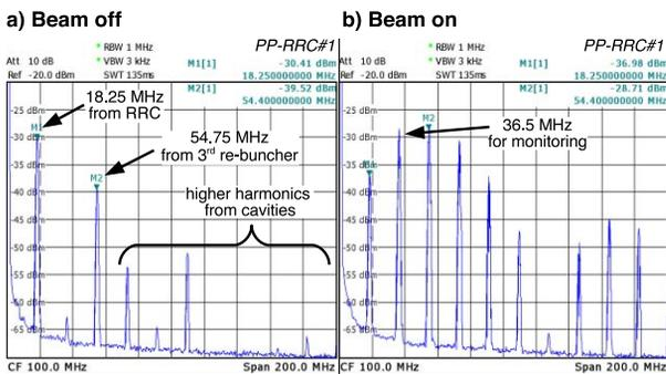
Figure 3: Frequency component of signal from PP-RRC#1 observed using spectrum analyzer under a) beam-off, and b) beam-on conditions.
