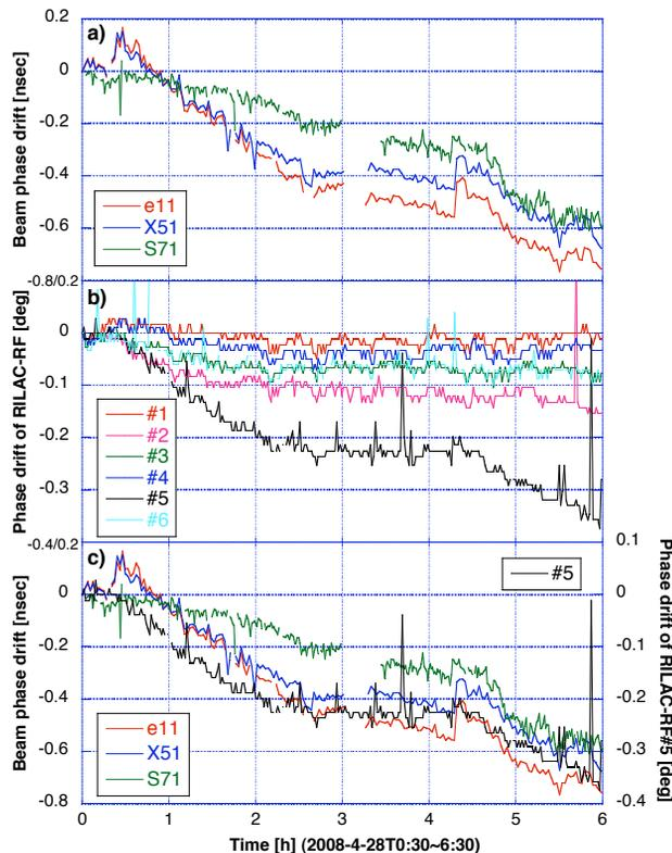
Figure 4: Phase drift of a) uranium beam, and b) RILAC-RF observed using developed SR844 systems. A correlation between RF phase of RILAC-#5 and beam-phases at PPs-e11, X51, and S71 was observed as shown in c).
