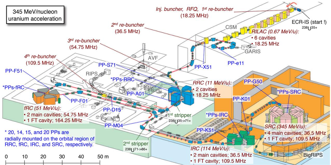
Figure 1: Layout of RIBF showing operational parameters for 345 MeV/nucleon uranium acceleration. The positions of phase probes (PPs) used for a beam-phase monitoring are also shown. PPs which are radially mounted on the acceleration region of cyclotrons (PPs-RRC, fRC, IRC, and SRC) are used for the tunings of isochronous magnetic field of cyclotrons.
