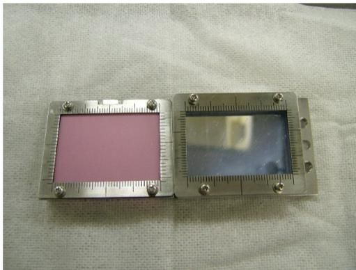
Figure 2: Screen folder mounted with both of a ceramic screen and a Cherenkov radiator. The left screen is a profile monitor with a fluorescence ceramic screen with a thickness of 0.1 mm and it is tilted vertically by an angle of  $45^\circ$ . The right screen is the aerogel radiator and it is tilted of  $55.8^\circ$ .
