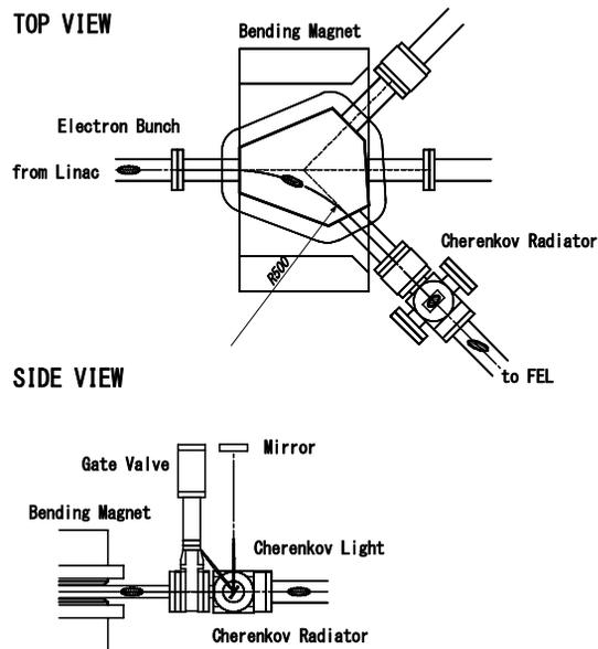
Figure 3: Configuration of the Cherenkov radiator.
