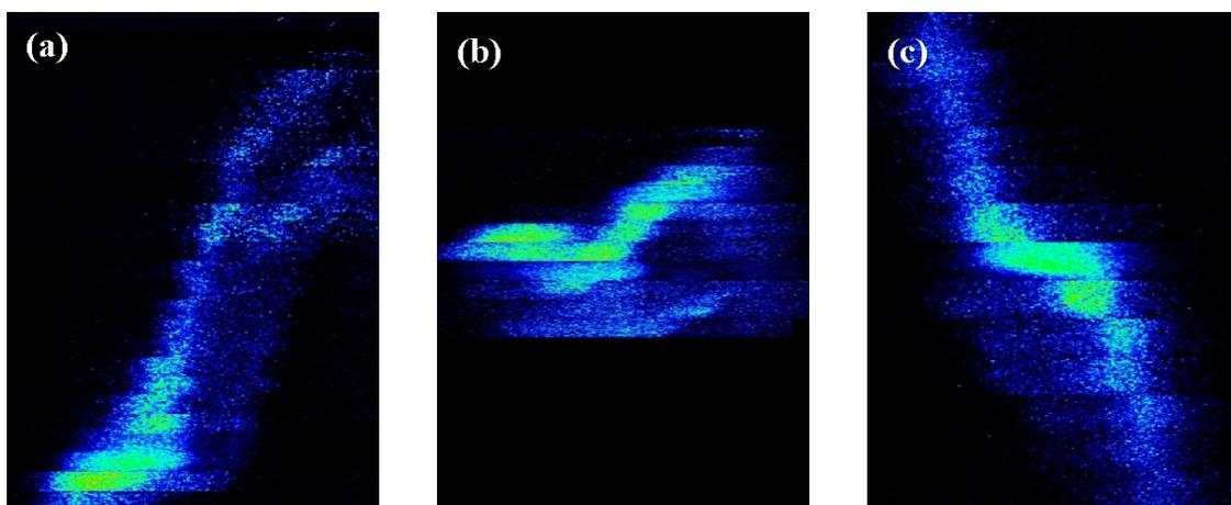
Figure 5: Reconstructed longitudinal phase-space profiles of the single bunch electron beam for three different accelerating phases. The profile images have temporal information as the horizontal axis (150 ps / full scale) and energy one as the vertical (9.6 % or 2.6 MeV / full scale). The left side indicates the head in the electron bunch. Accelerating phases of the bunch center are estimated to (a)  $-20^\circ$ , (b)  $-10^\circ$  and (c)  $0^\circ$  from the rf crest, respectively.
