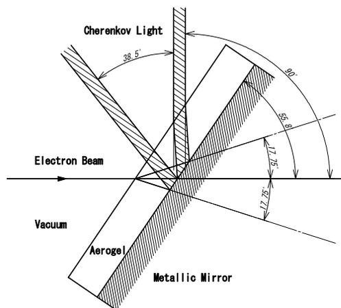
Figure 1: Schematic design of the Cherenkov radiator.
