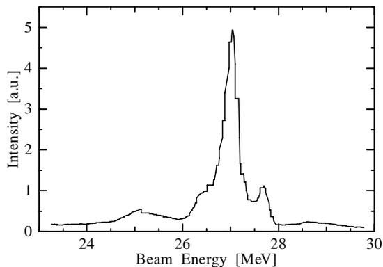
Figure 4: Energy spectrum of the single bunch electron beam with the peak energy of 27 MeV and the total charge of 30 nC.
