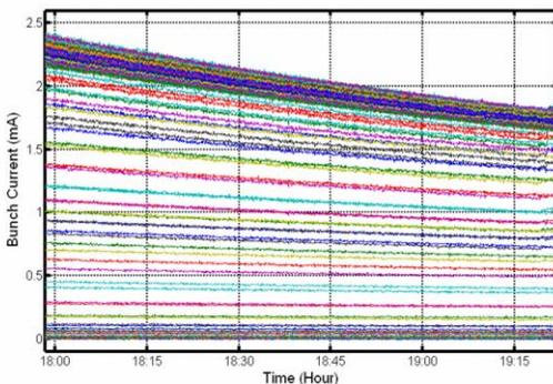
Figure 3: Bunch current decay during one hour period.
