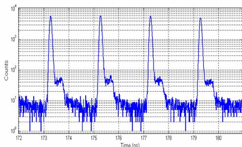
Figure 8: Filling pattern measured by the TCPCS. The vertical axis is in log scale.
