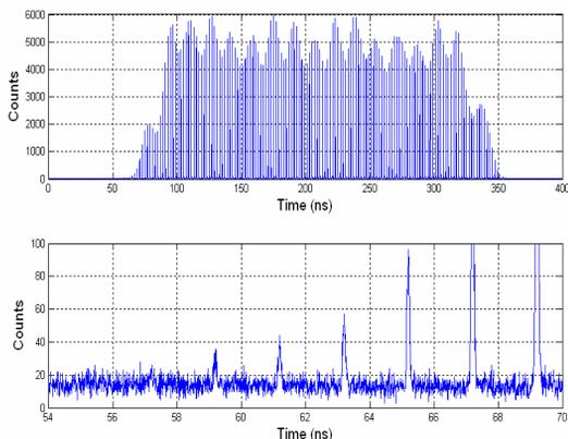
Figure 7: Filling pattern measured by the TCSPC. Vertical scale is in linear scale. The stored beam current is 301 mA. The above figure is the filling pattern of the whole ring, the below figure show very small bunches existed at the leading fringe of the major bunch train.
