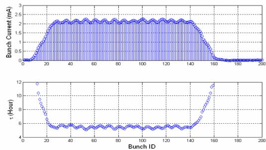
Figure 4: The above figure is shown the bunch population distribution at the instance for lifetime calculation. Distribution of the bunch lifetime is shown in the below figure.
