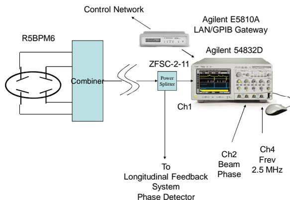
Figure 1: Pickups based bunch current measurement system.
