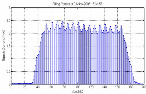
Figure 2: Measured bunch current of a snapshot during top-up operation. Total beam current is 302 mA.
