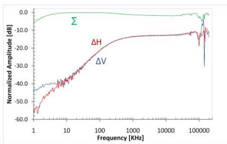
Figure 5: Frequency response of the BPS signals.
