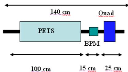
Figure 1: Schematic of a TBL cell.
