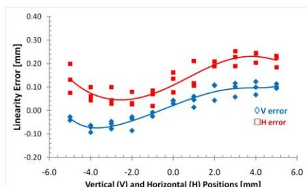
Figure 6: Linearity error for both planes.
