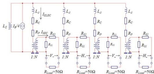
Figure 4: Low-frequency electrical model.
