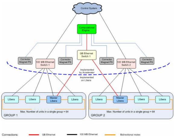
Figure 2: Libera Grouping and fast orbit feedback topology.
