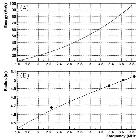
Figure 3: Calculated (A) beam energy and (B) radius at a center of a straight section as functions of revolution frequency; Symbols show the measured values.
