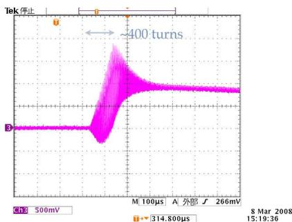
Figure 5: Beam accumulation and survival in the FFAG ring.
