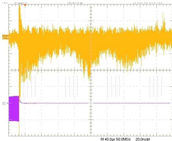
Figure 2: Output signals from bunch monitor of the main ring (yellow) and the booster (magenta); 40  $\mu$ s/div.
