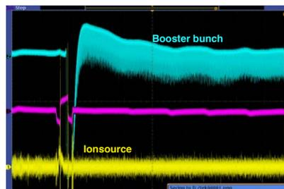
Figure 1: Output signal from current transformer (CT) right after the ion-source (yellow), and Booster bunch monitor (blue); 100 ms/div.
