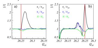
Figure 2: Octupolar resonance: a) Space charge induced emittance increase and beam loss; b) Electron cloud induced emittance increase and beam loss. (38 kicks per betatron wavelength and synchrotron. motion included).
