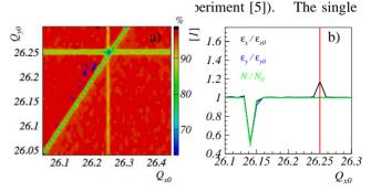
Figure 1: a) Resonance lines excited by a single octupole; b) Emittance growth and beam loss for several tunes at  $Q_{y0} = 26.1$ .
