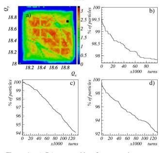
Figure 4: a) DA scans with reference random errors. Black marker: proposed working point WP1; b) Beam2 for the standard error case; Beam loss with space charge for Beam1 c) and Beam2 d) for an intensity of  $3 \times 10^{11}$  ions.
