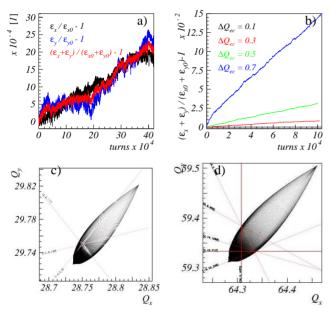
Figure 5: a) RHIC beam emittance evolution versus turns for  $\Delta Q_{ec} = 0.03$ ; b) LHC beam emittance evolution versus turns for  $\Delta Q_{ec} = 0.1$ ; c) Frequency map for RHIC for a beam with  $\Delta Q_{ec} = 0.1$ ; d) Frequency map for LHC for a beam with  $\Delta Q_{ec} = 0.1$ .
