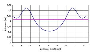
Figure 2: thickness variation along half chamber profile.
