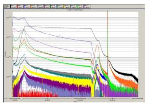
Figure 7: RGA during bake-out and NEG activation.
