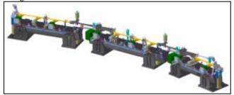
Figure 5: Typical SOLEIL's cell lay-out. NEG coated q-pole chambers are in yellow.
