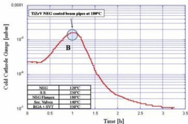
Figure 3: Pressure variation during the activation of the TiZrV NEG coated beam pipes.
