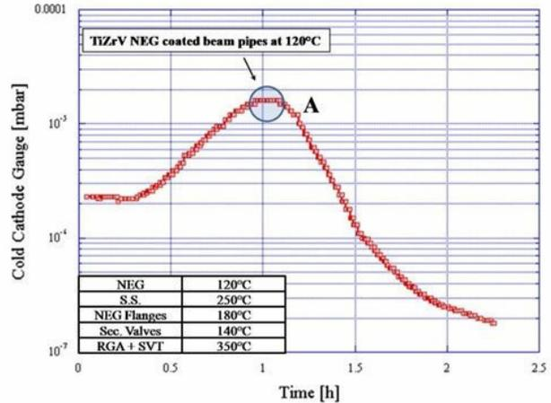
Figure 2: Pressure variation during the bake-out cycle.
