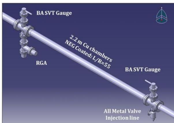
Figure 5: Schematic draft of the vacuum pilot sector.
