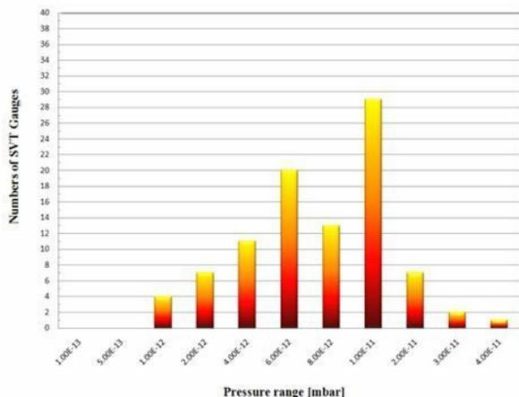
Figure 4: Ultimate pressure distribution on the TiZrV NEG coated beam pipes after activation.
