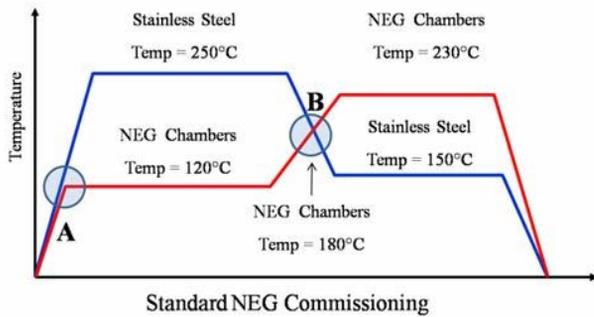
Figure 1: Schematic of the bake-out/NEG activation cycle of the TiZrV NEG coated beam pipes.
