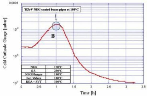
Figure 3: Pressure variation during the activation of the TiZrV NEG coated beam pipes.
