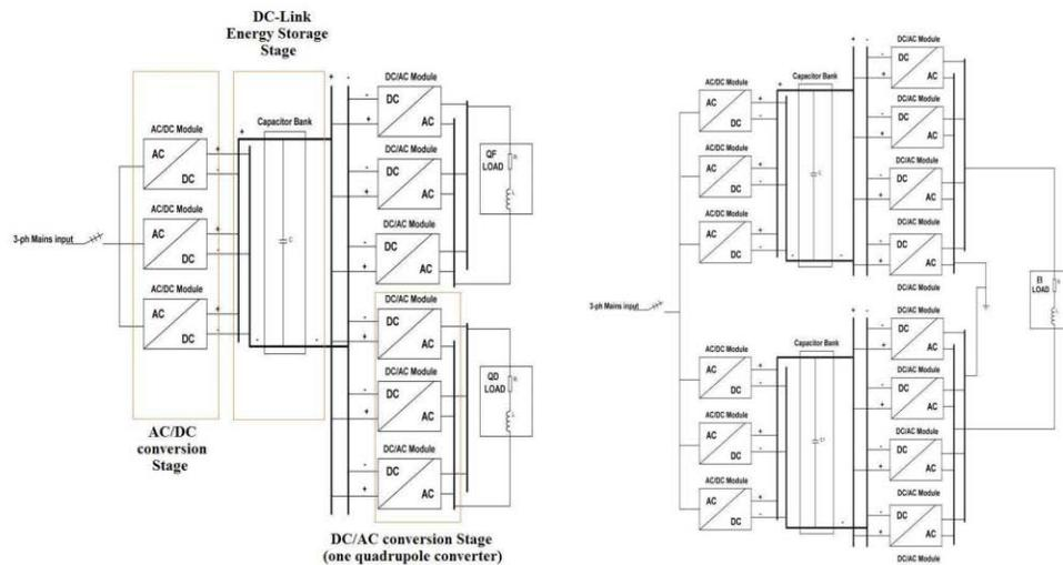
Figure 2: Structure of the Quadrupole (left) and Dipole (right) Power Converters.
