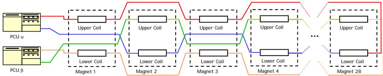
Figure 1: Dipole magnets connections (PCU – Power Converter Unit).
