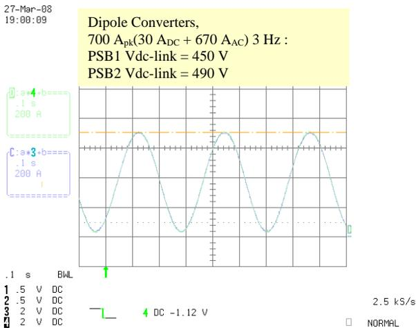
Figure 6: Measured current waveforms from the dipole converters at nominal frequency and peak current (the two traces are overlapped).
