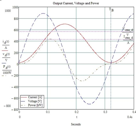
Figure 5: Example of output waveforms for each dipole power converter.
