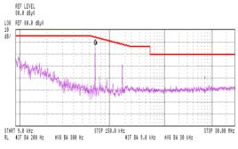
Figure 2: EMC measurements of an LHC power converter.
