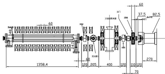
Figure 3: Buncher section.
