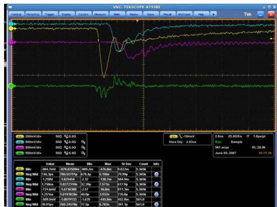
Figure 5: the beam waveform when the sub-harmonic cavity does not operate.
