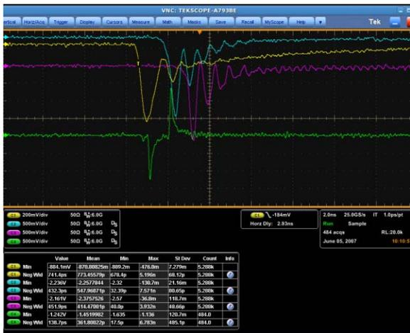
Figure 6: the beam waveform when the sub-harmonic cavity operates
