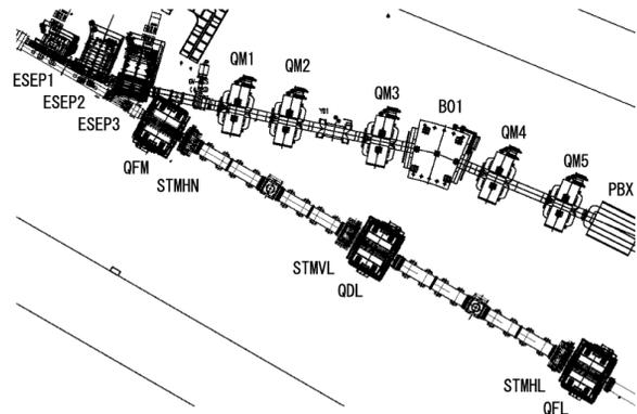
Figure 4: The schematic diagram of the RCS extraction area.
