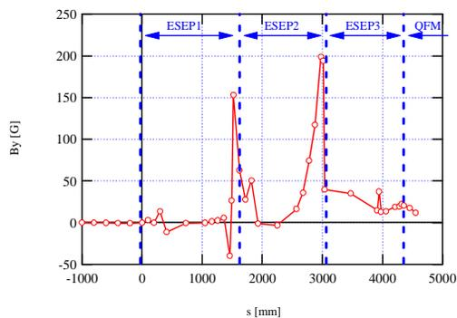
Figure 5: Measured leakage field distribution from the ESEPs along the s-axis on the top of the vacuum chamber, in which the origin of s-axis indicates the upper-stream flange of the ESEP1.
