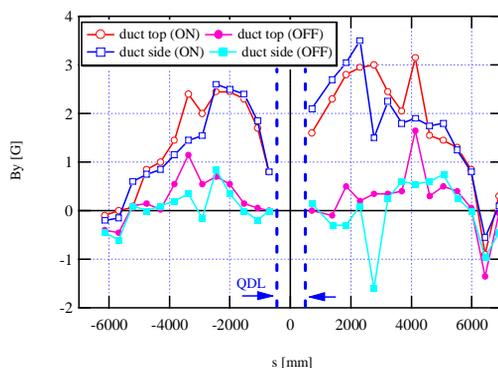
Figure 6: Measured field distribution leaked from the 3NBT-B01 along the s-axis on the top and side of the vacuum chamber, in which the origin indicates the center of the QDL.
