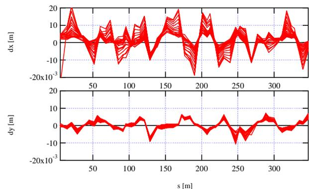
Figure 1: Measured closed orbits as a function of the longitudinal distance during the acceleration from 181 MeV to 3 GeV, in which the upper one shows horizontal closed orbits and the lower one shows vertical ones.
