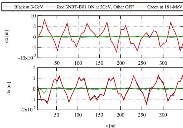
Figure 3: Measured CODs caused by the 3NBT DC magnets at injection energy. The COD with each operation pattern of the 3NBT DC magnets is compared to COD with all DC magnet off, in which the upper one shows horizontal closed orbits and the lower one shows the vertical ones.
