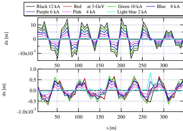
Figure 2: Measured CODs caused by the ESEPs at injection energy. The COD with each exciting current of the ESEPs is compared to COD with all DC magnet off, in which the upper one shows horizontal closed orbits and the lower one shows the vertical ones.
