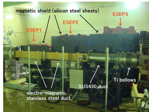
Figure 7: Three extraction septum magnets installed in the RCS tunnel.
