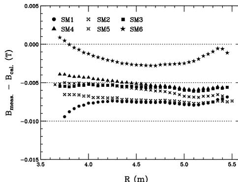
Figure 3: The deviation of average magnetic field of each sector magnet at the main coil current of 5000 A.
