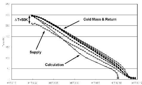
Figure 2: Cool-down curves of the SRC superconducting magnets.
