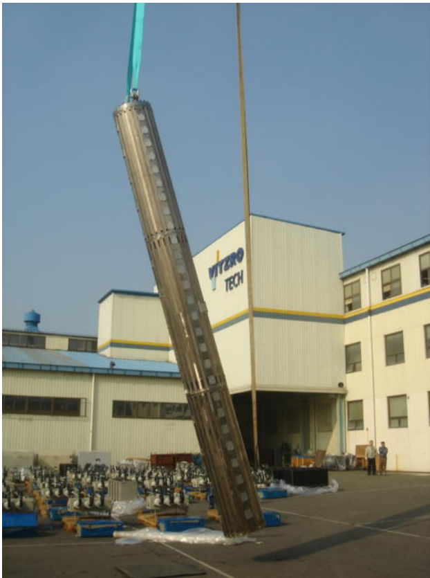
Figure 2: 3-section combined into one tank assembly.
