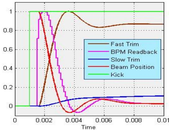
Figure 5: Response of the integrated orbit feedback system to the step.
