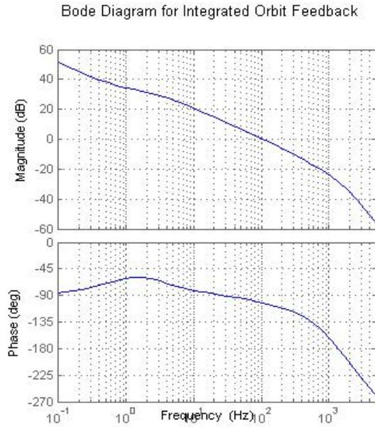
Figure 3: Bode diagram of integrated orbit feedback.
