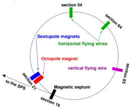
Figure 1: Schematic layout of the PS ring with the elements used during the experiments.
