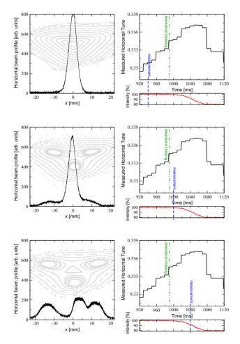
Figure 2: Evolution of the horizontal beam profile during the crossing of the one-third resonance. The profile is shown before the resonance is crossed (upper), right after the crossing (centre), and at the end of the crossing (lower). The corresponding phase space portrait obtained from the MADX PS model is superimposed to the measured profile. 05 Beam Dynamics and Electromagnetic Fields
