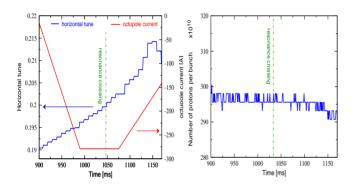
Figure 4: Left: measured horizontal fractional tune and time evolution of the octupole current in the interval where the one-fifth resonance is crossed. Right: number of protons per pulse measured by the current transformer.
